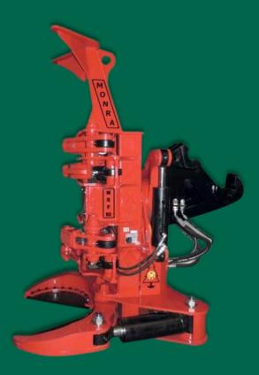
The Monra MRF-60 cutting head is characterized by its great performance, capacity and the use of high-quality materials for manufacturing. This all results in its great robustness and reliability. It's designed to perform demanding, continuous work safely and easily. It is ideal for felling any type of tree. Adapts to any base machine on the market from 20 tons.
